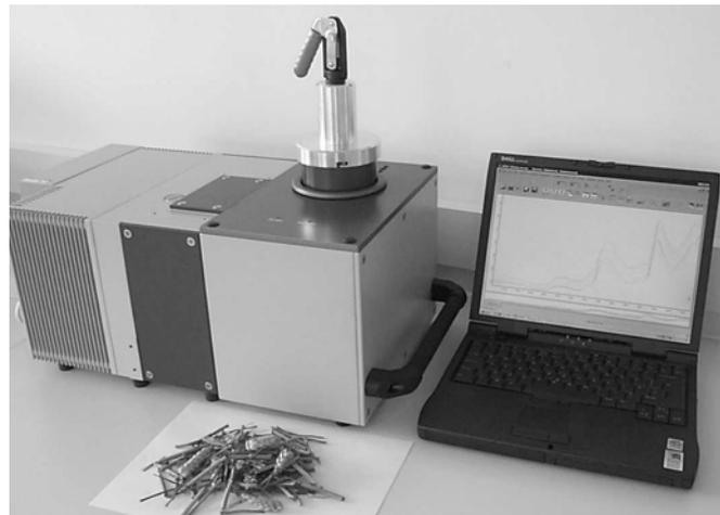
**Figure 4. The laboratory-based Vector 22/N-I FT-NIR instrument**
