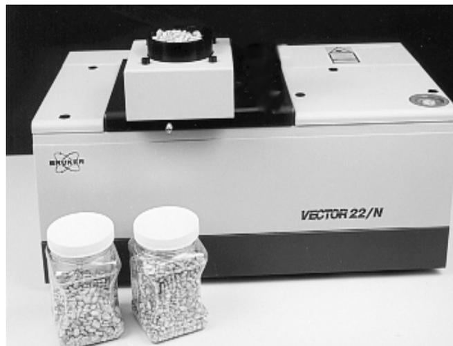
**Figure 5. The rotating sample cell and integrating sphere detection assembly**
