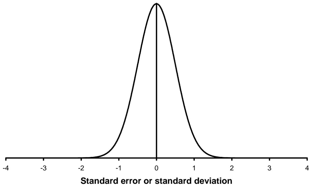
**Figure 13. Comparison of the distribution of errors for a population having a standard deviation of 1 and that of an NIR calibration having a standard error of 0.5. The means of the two distributions differ.**
